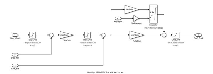
The tutorial uses model RollAxisAutopilotHarness to test RollAxisAutopilot.
